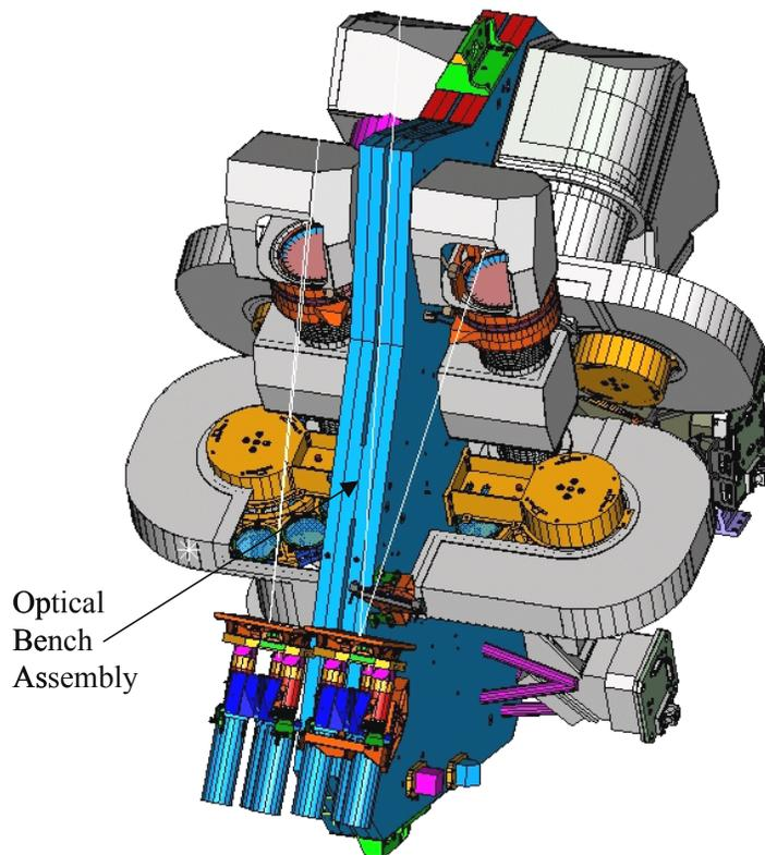
Figure 1: NIRC*am* Instrument with back to back optical modules supported by two optical benches
