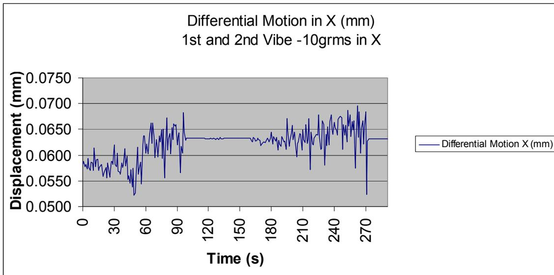
*Figure 13 – Decentration results for vibration of the dummy lens cell assembly*
