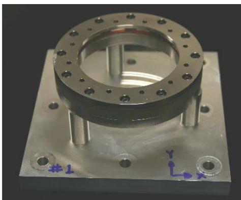
Figure 10 – The test fixture for the 12-pad vibration test
