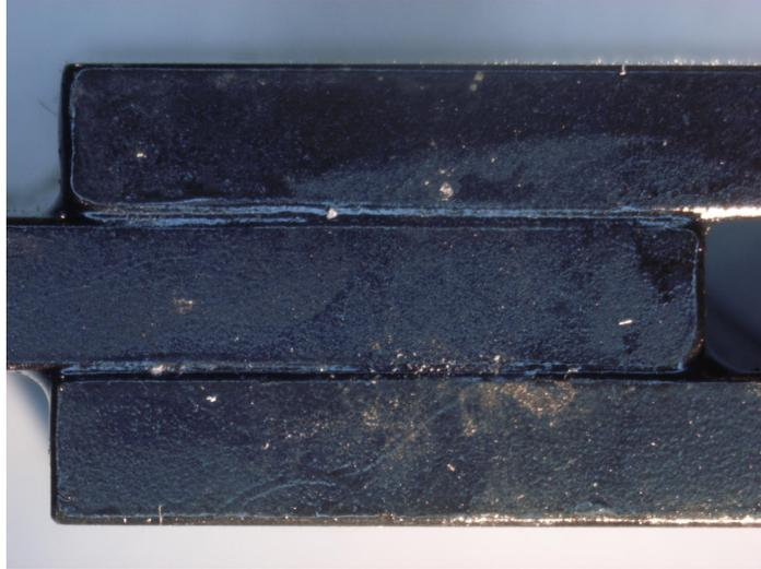
Figure 5. Anodized and Primed Bond Coupon
