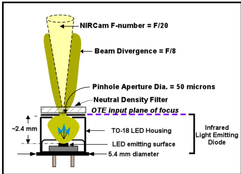
Figure 12. Point source design with pinhole aperture and neutral density filter
