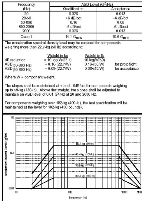
Figure 7 – Vibration test spectrum from GEVS (ref.
