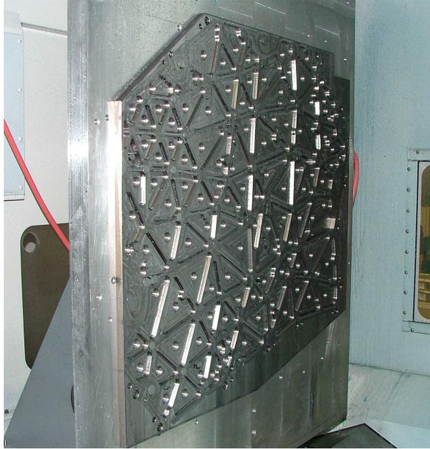
Figure 8. NIRCam I-220H During Machining
