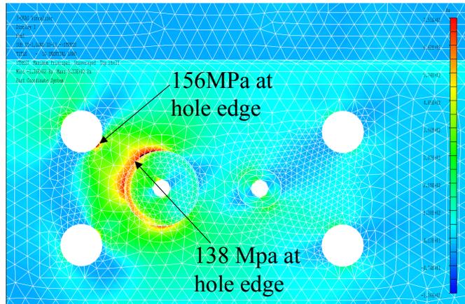
Figure 10: Local Stress with Left Lateral Load
