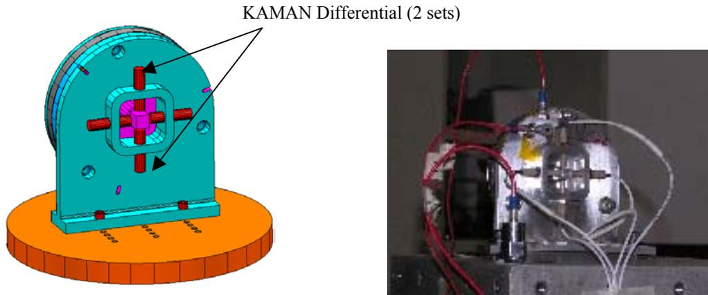
*Figure 12 – KAMAN differential sensor set-up with lens dummy and photo of actual set-up*
