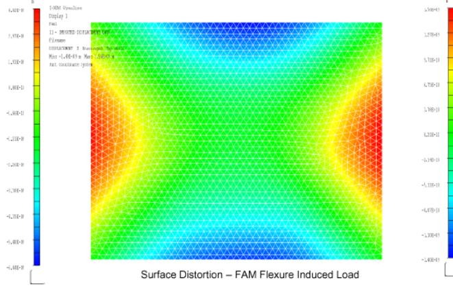
Figure 8. FAM Flexure Induced Load (< 2nm full scale)
