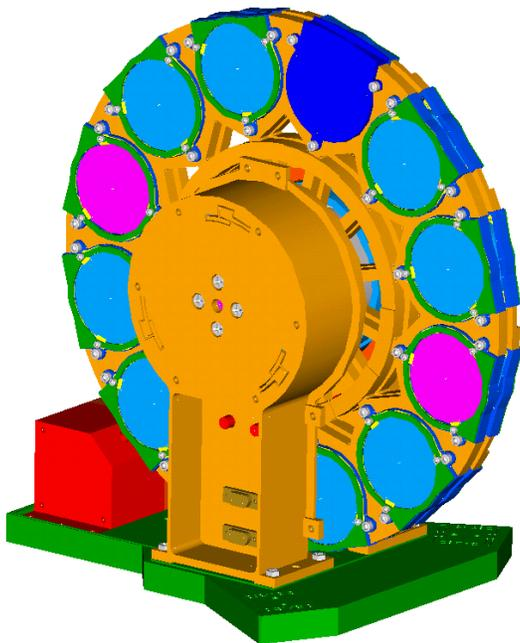
Figure 7. Filter Wheel Assembly (FWA)
