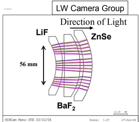
Figure 2. NIRCam Triplet Lens Assemblies
