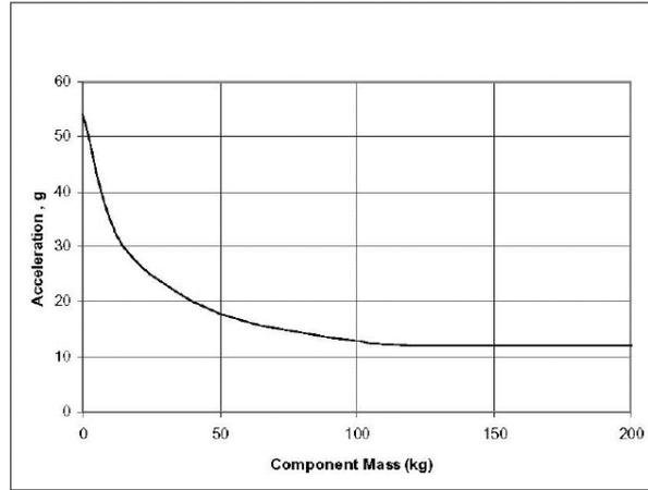
Figure 6 – Mass acceleration curve relevant to NIRCam
