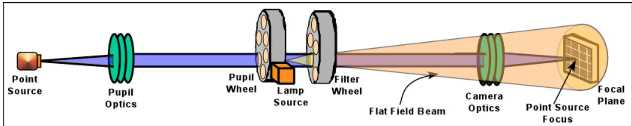
Figure 1. Location of NIRCam Calibration Sources
