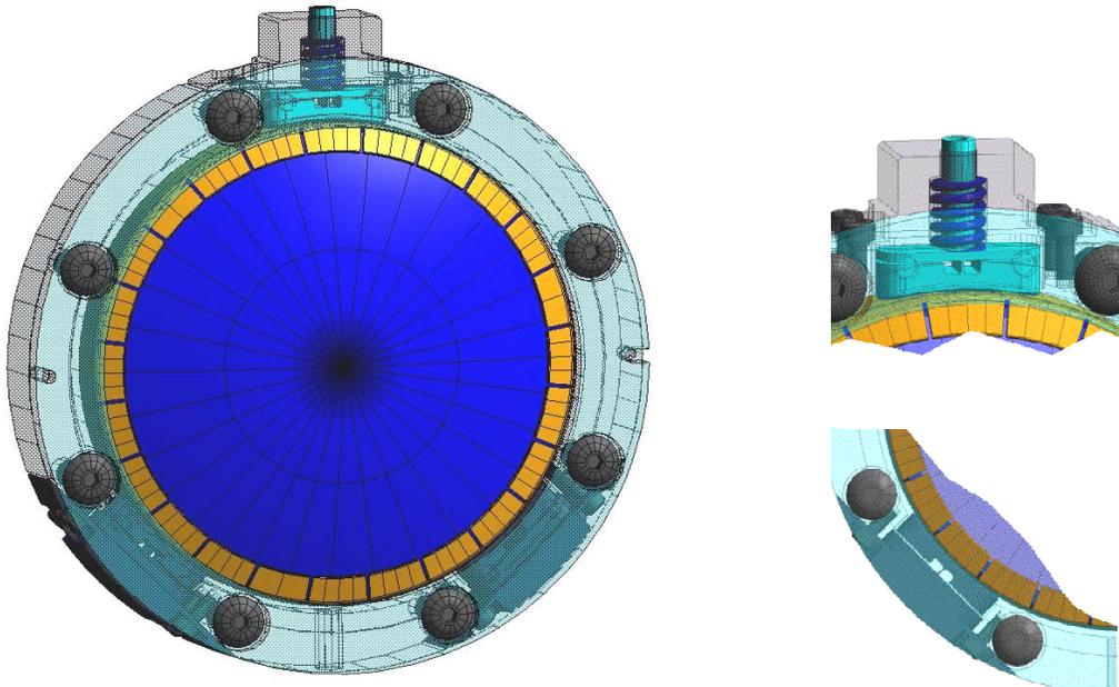
Figure 2 – Original 3 pad flexure design at left. At right, the spring loaded plunger and flexured pad (2places).
