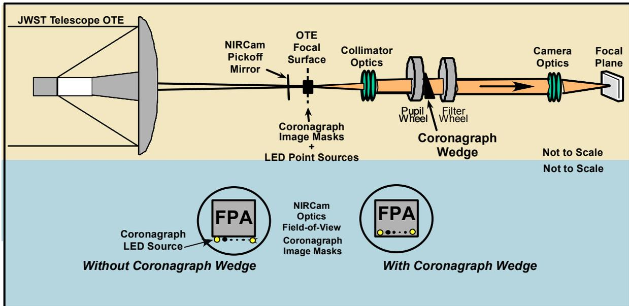
Figure 9. Relative locations of LED Point sources with respect to NIRCам optical train.
