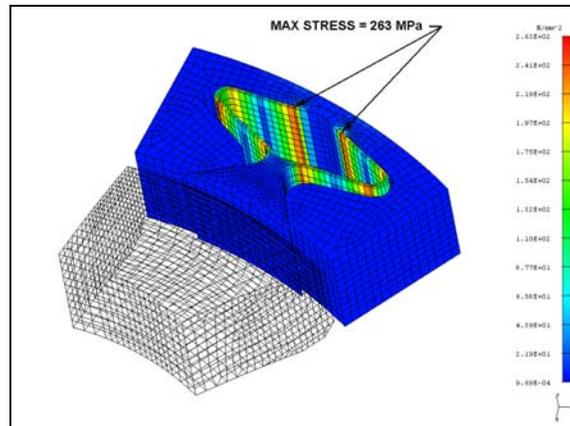
Figure 9 - Titanium Flexure Maximum Stress
