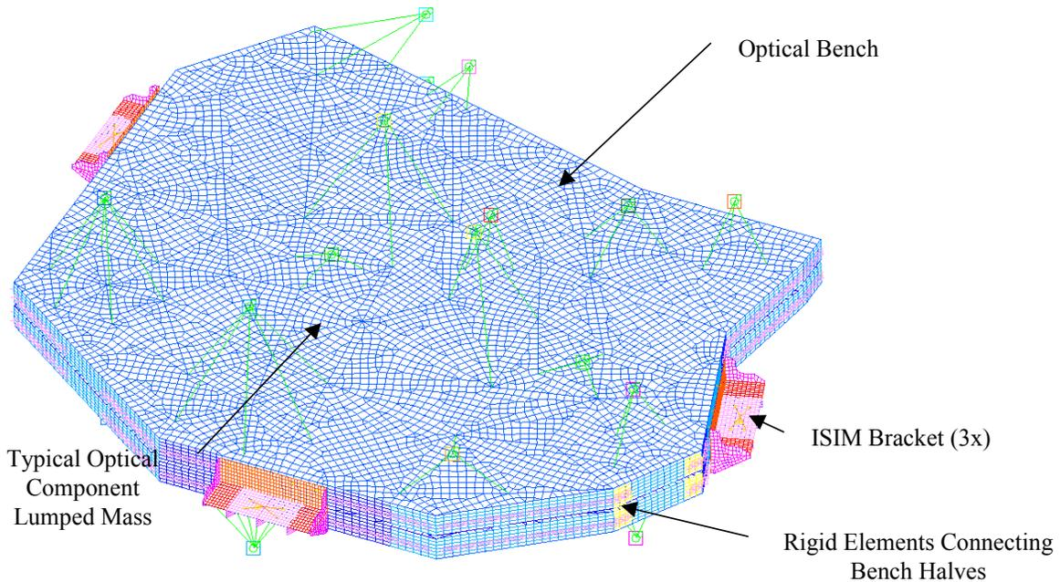
Figure 7: Optical Bench Assembly finite element model
