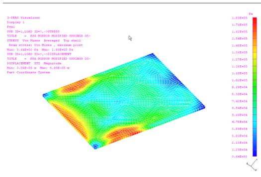
Figure 16. 54G Shock stress on mirror is 0.18 MPa maximum
