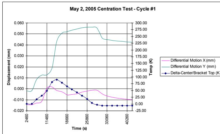
Figure 15 First Cryo-cycle data
