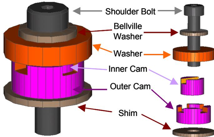
Figure 5: Component attachment method providing adjustability
