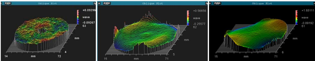
Figure 3 – In the left image is a ZYGO surface map of the LiF optic as received by the vendor. Total rms WFE = 0.012 waves at  $\lambda=633\text{nm}$ ; 0.186 wave P-V. The middle image shows the optic after having been mounted, and then removed from the mount. Clearly there is already distortion evident in the optic with rms WFE = 0.073 wav; 0.822 P-V. The right image shows the optic unmounted after vibration. Many waves of distortion at the radial mount points that were off-scale.
