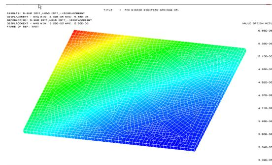
Figure 17. Bulk cool down surface displacement is less than 300 nm corner to corner
