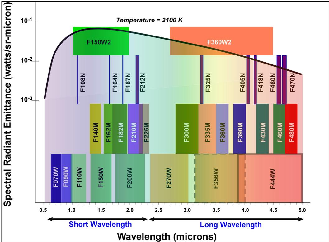
Figure 7. Absolute spectral radiance (Watts/sr-micron) for type 715 tungsten lamp, superimposed on NIRCam filters
