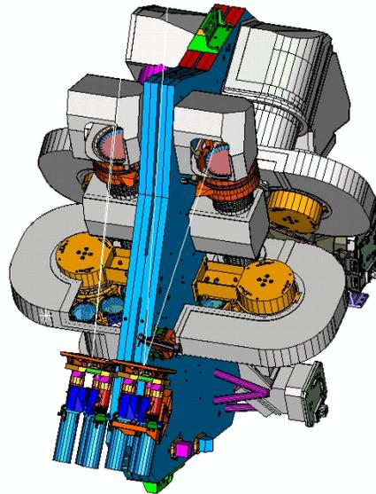
Figure 4. NIRCcam focal plane array coverage on the sky      Figure 5. A side and B side NIRCcam imager modules
