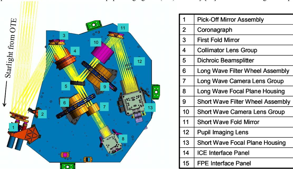
Figure 1. Short-wave and long-wave channels in a NIRCcam imager module. An identical module is on the back side.
