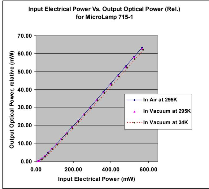
Figure 6. Input electrical power versus output optical power for air at 295 K, vacuum at 295 K, and vacuum at 34 K.
