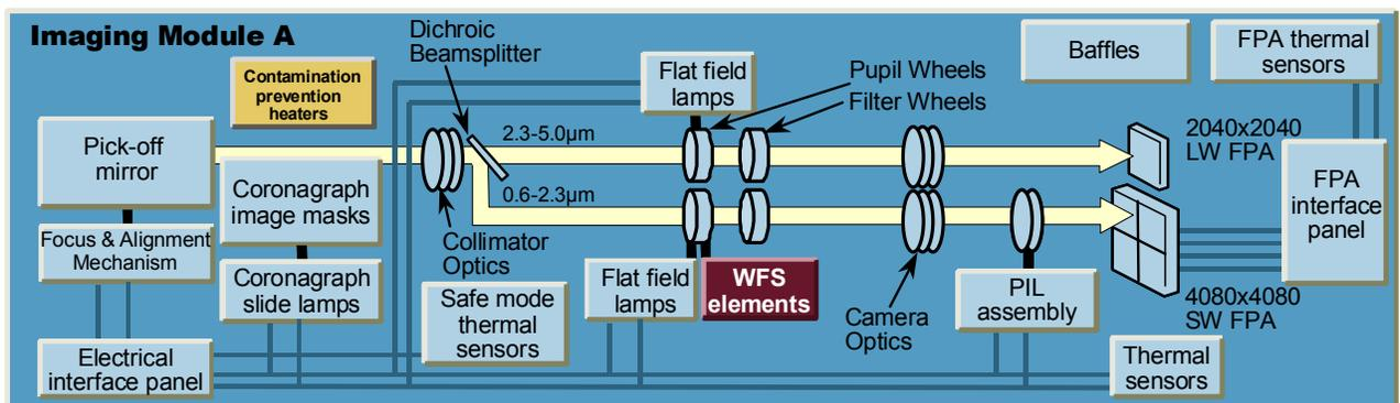
Figure 3 Short-wave and long-wave channels in a NIRCam imager module
