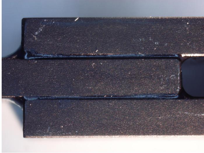
Figure 3. Anodized Bond Coupon
