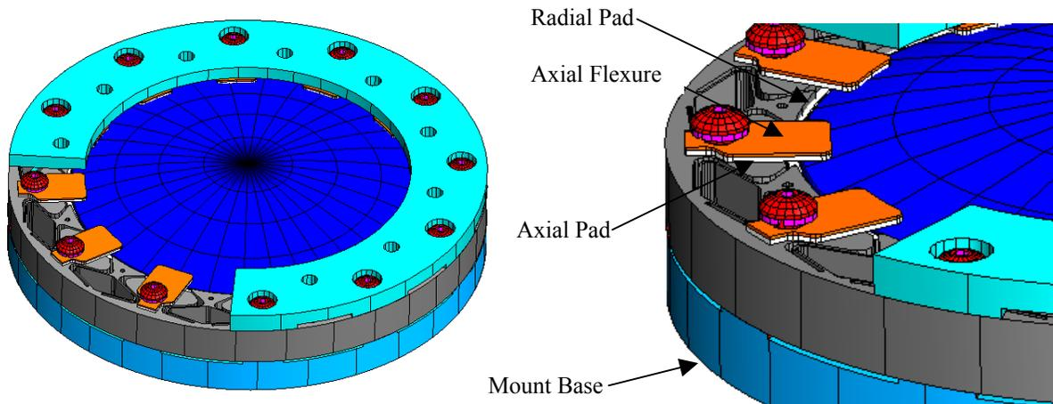
Figure 5- Lens cell cutaway and detail of axial and radial flexure and pads
