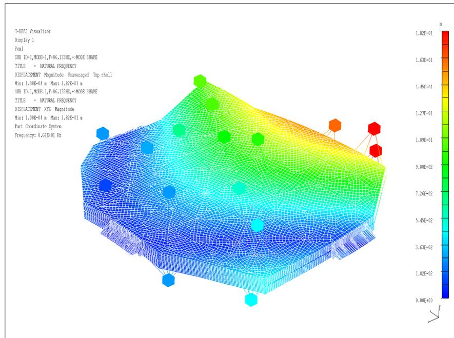
Figure 9: First Mode at 86 Hz (scale is greatly exaggerated)
