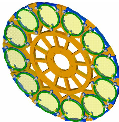
Figure 3: The NIRCcam Filter Wheel accepts 12 optical elements
