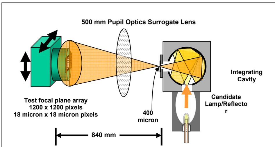
Figure 4. Flat field spatial distribution measured with integrating cavity and camera
