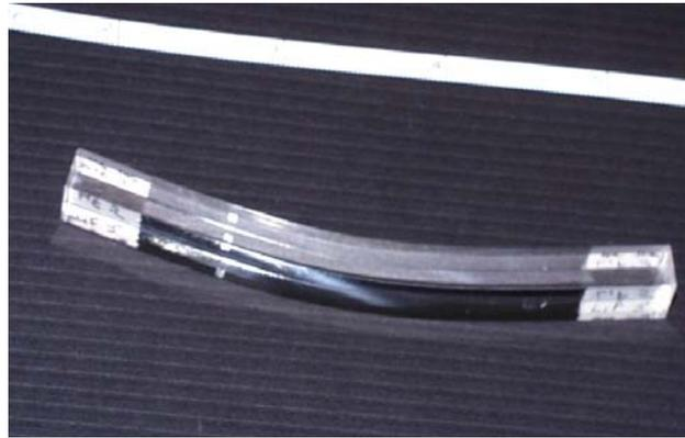
Figure 1 – LiF specimen (90mm X 8mm X 6mm) yielded after 4-point bend test
