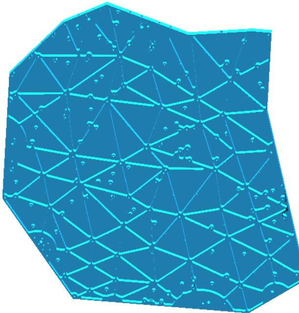
Figure 3: Optical bench internal rib geometry
