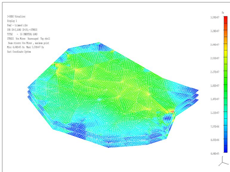
Figure 8: Bench Stresses peak at 36 MPa with a 12g Load applied Perpendicular to the Bench
