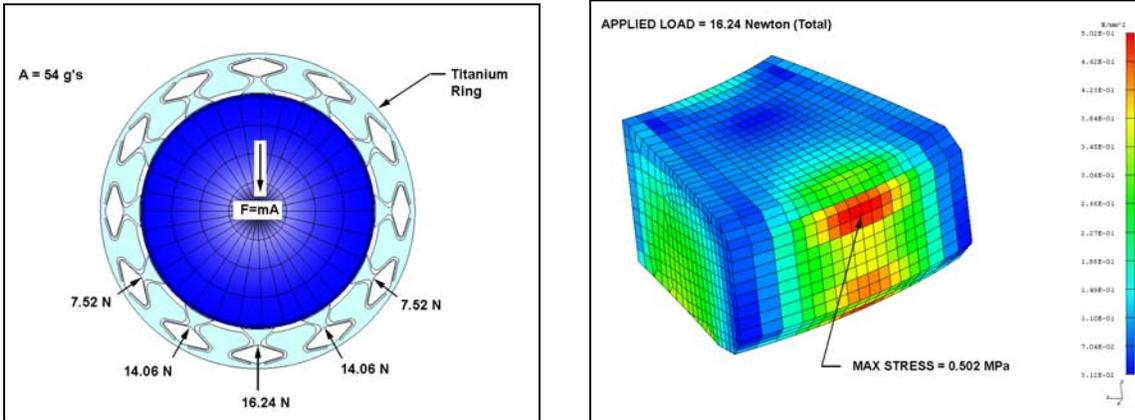
Figure 8 Lithium Fluoride Lens Max Stress due to Applied  $F = 16.24$  Newtons
