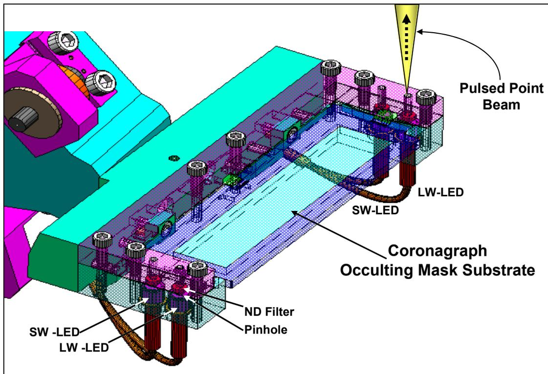
Figure 10. Coronagraph Occulting Image Mask mounting fixture with LED point source projectors
