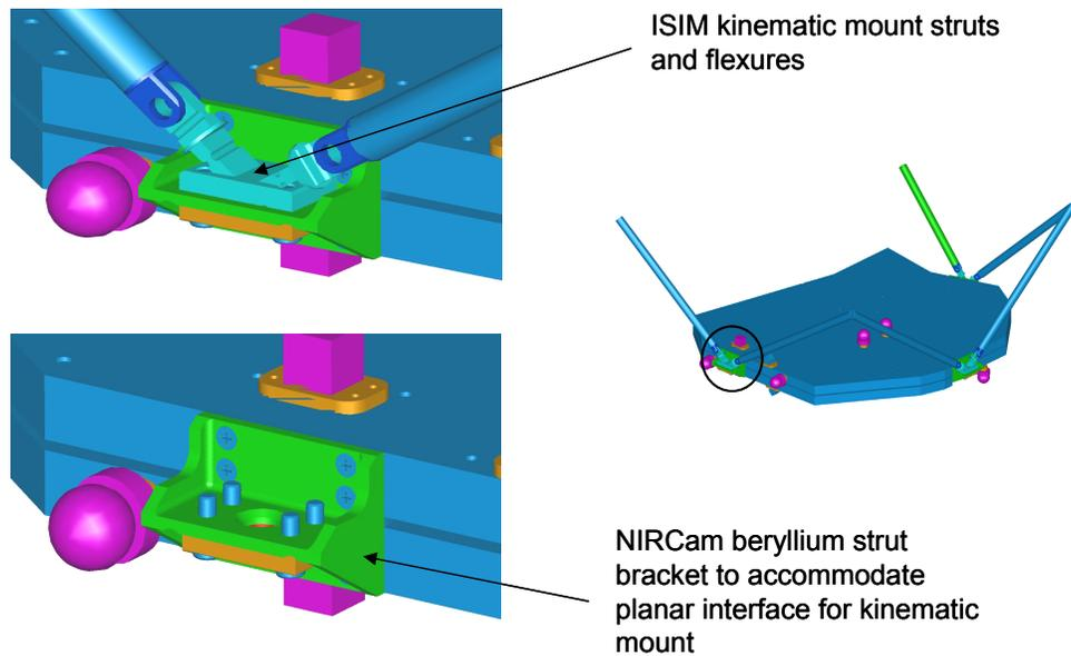
Figure 6: ISIM Interface brackets with struts attached
