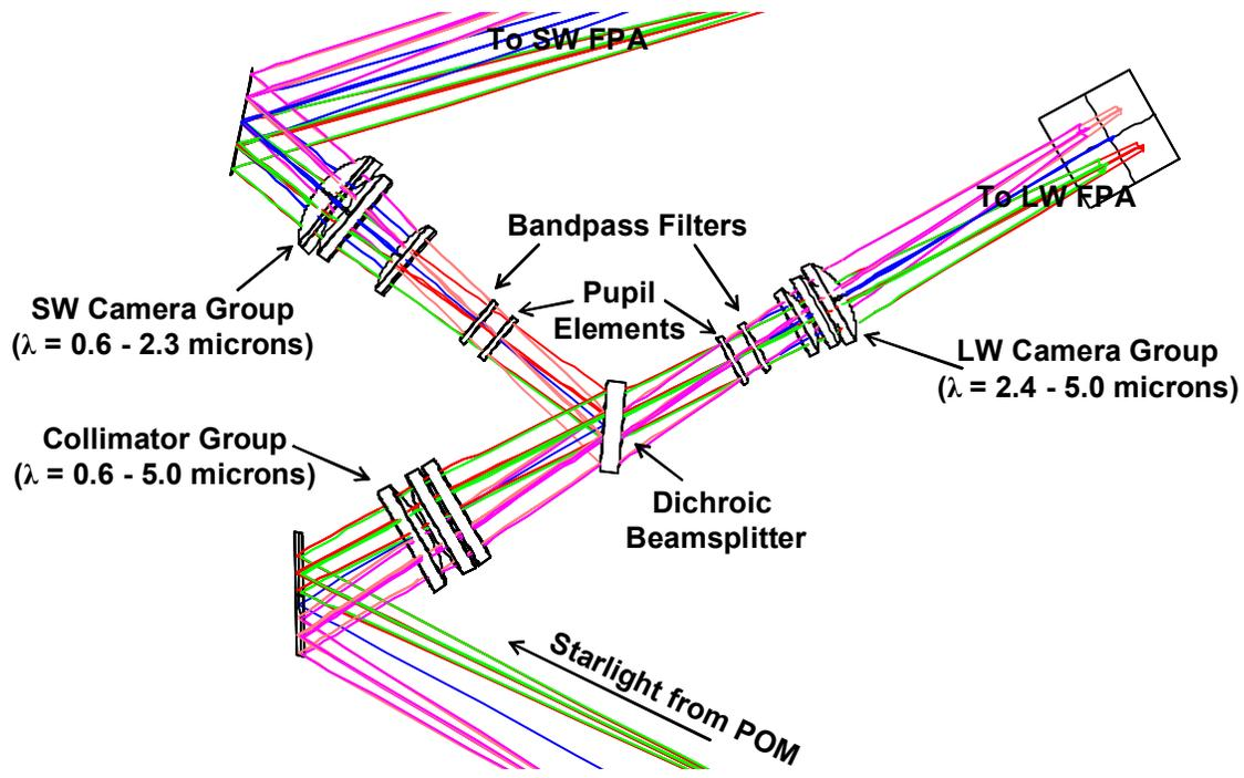
Figure 6. Schematic Diagram of the short wave and long wave optical paths within a NIRCam imager module
