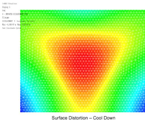
Figure 7. Cool Down Distortion (< 2nm full scale)
