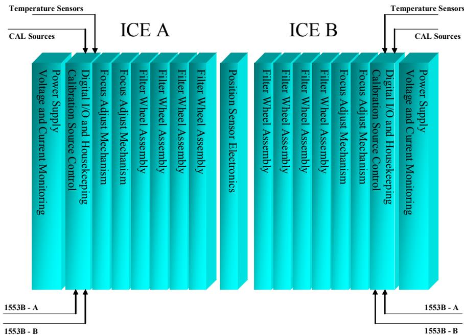
Figure 13. NIRCcam Instrument Control Electronics
