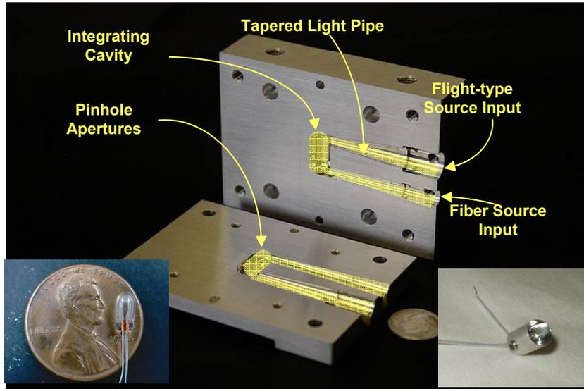
Figure 3. Gold coated integrating projection cavity. Test version.
