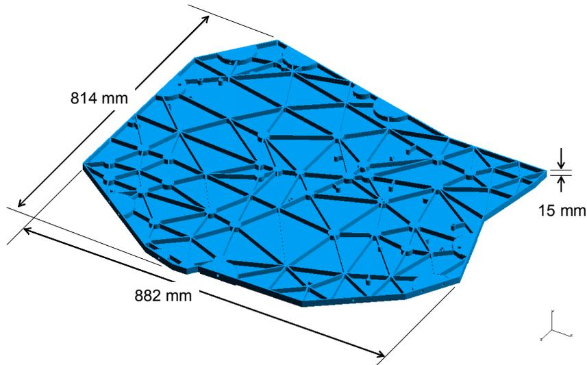
Figure 10. Optical Bench Assembly (OBA) imager module half-plate
