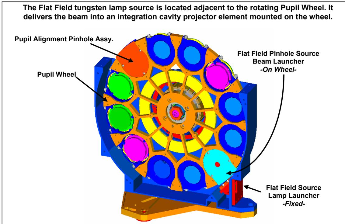
Figure 2. Flat Field Projector mounted on rotating Pupil Wheel. Adjacent source on fixed bench.
