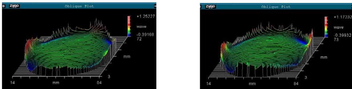
Figure 11 – Comparison of the surface maps for the LiF optic pre and post vibration in the 12 pad diamond flexure mount. The pre-vibe plot is on the left; rms WFE was 0.128 waves, 1.644 waves P-V. The post vibephot is on the right; rms WFE value was 0.134 waves, 1.572 P-V. Note that the optical quality prior to vibrate for this optic was not as good as the optic vibrate in the original mount.
