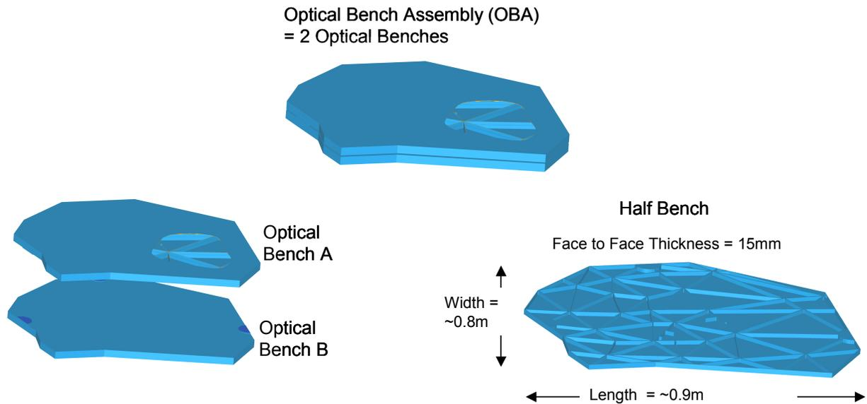
Figure 2: Optical Bench Assembly configuration showing a portion of the facesheet removed to show the internal rib structure.
