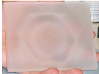
Figure 3. Pick Off Mirror (Uncoated)
