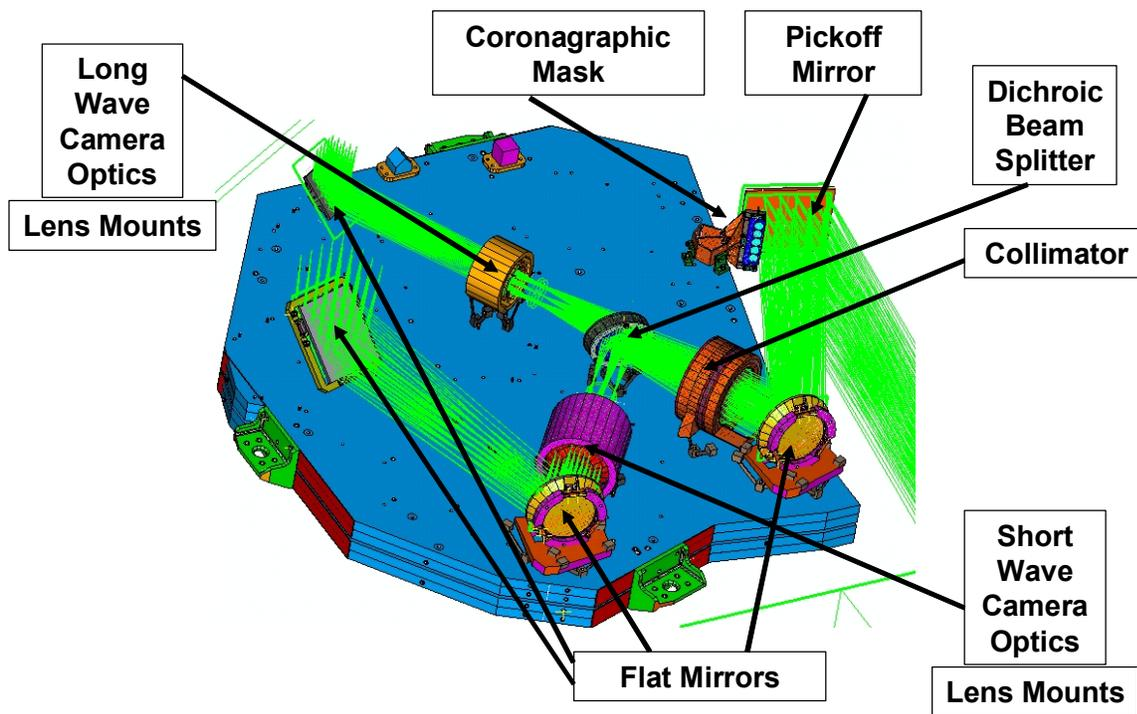
Figure 9. Imager optical train on the optical bench
