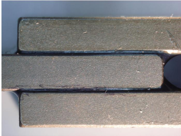
Figure 4. Etched and Primed Bond Coupon
