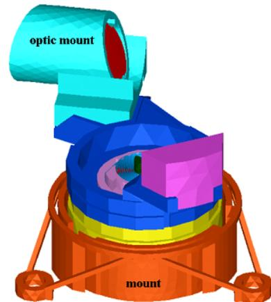
Figure 8. Pupil Imaging Lens (PIL) Assembly
