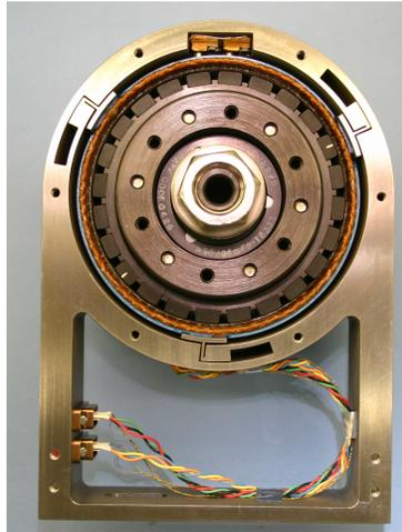
Figure 8: Filter Wheel Assembly Prototype
