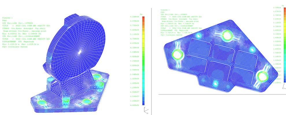
Figure 13. Bulk Cool Down Thermal Stresses peak at 40 to 50 MPa at the mounting holes
